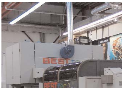
Figure 3: Reggiani DReAM printer being used in large-scale flag production in Berlin, Germany.
