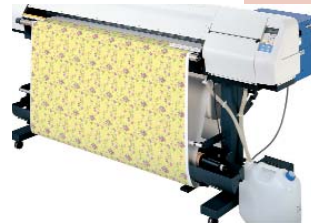
Figure 6: The DReAM industrial digital textile printer from Reggiani, capable of printing 86 inch-wide fabrics at 185 square yards per hour (1650 square feet/hour) at 600 dpi resolution.
