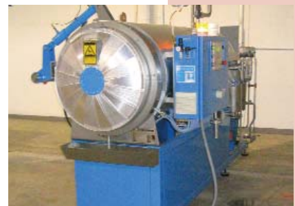
Figure 8: Xorella MINICONTEXXOR® for Fabric Steaming and Conditioning. For the use of all thermal treatments of fabrics of all substrates, both manmade and natural fibers within the saturated steam range between 50° - 150°C, for processes of print dye fixation. Handles fabrics up to 84 inches in width.
