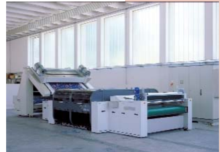
Figure 6: The DReAM industrial digital textile printer from Reggiani, capable of printing 86 inch-wide fabrics at 185 square yards per hour (1650 square feet/hour) at 600 dpi resolution.
